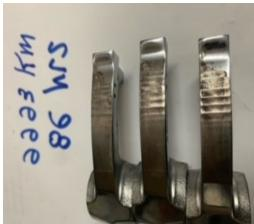
something like this. The picture **left** is a part of a set from a unit that has approximately 2200 Km (1300 miles) on it. We expect that the worn surface could be caused by two separate reasons. We are of the opinion that the structure of the stock flyweight helps start the problems.
